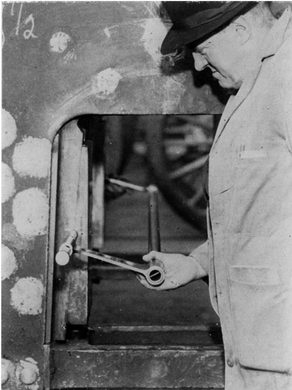
Fig. 18A. Application of overall frame and horn edge width gauge.
