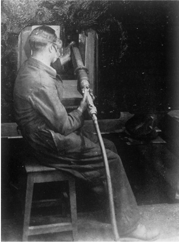
Fig. 6. Rod-type pneumatic grinder.
