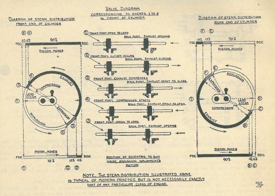
WHEN considering the steam cycle within the cylinder, the position of both piston and crank must be taken into account, because the duration of the various "periods" in the working cycle are measured in terms of the piston stroke or angular movement of the crank, whilst the complete cycle embraces one revolution of the crank or two strokes of the piston.
