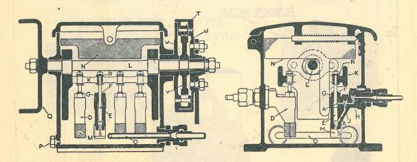
the purpose of replenishing the oil which is filtered through a large fine mesh sieve N.
