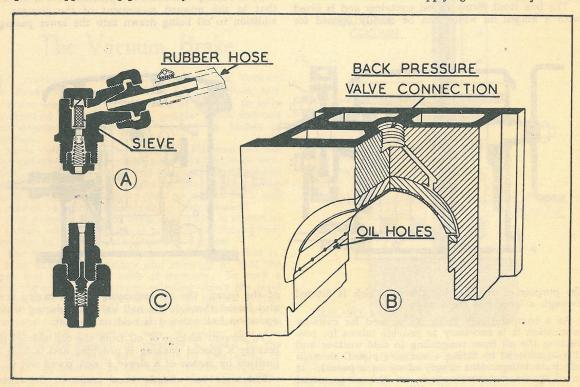
This difficulty is, however, overcome by terminating the copper pipe in a union connection fixed rigidly to the frame at a point conveniently near the axlebox, the final connection being made with a short length of specially prepared armoured rubber hose.
