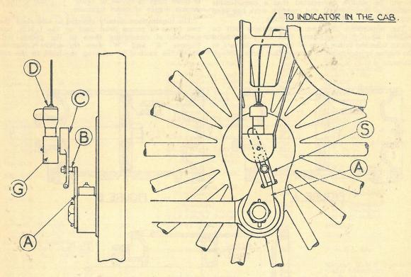
THE strict observance of speed restrictions is of the utmost importance, and in order to assist drivers speed indicators have now been fitted to a number of express passenger engines.
